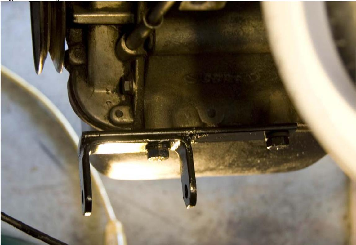
Figure 3. *The bracket on the block.*
