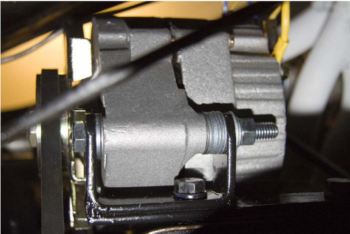
Figure 4. *The alternator installed with steel and thinner stainless steel washers for shims.*
