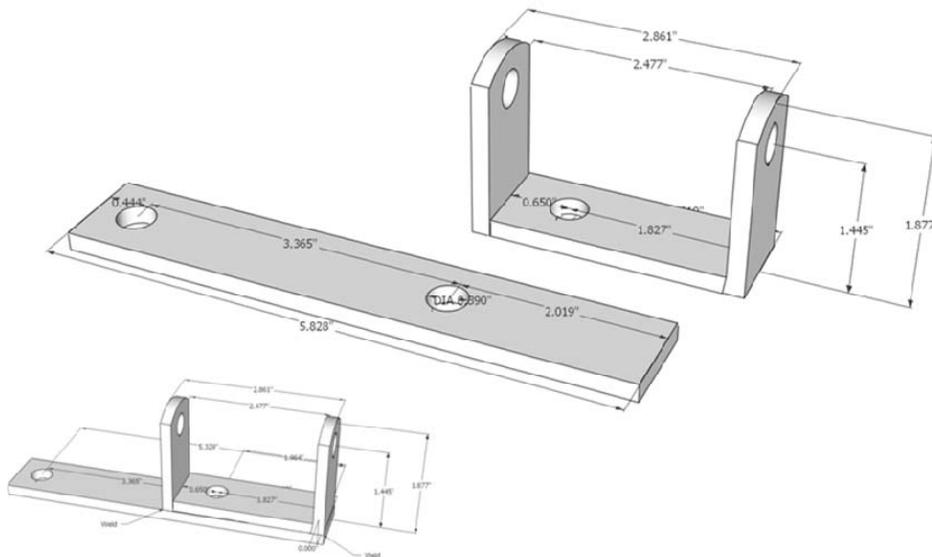
**Figure 1. Bracket for GM alternator on Ford 1500 (should fit any Kent engine)**
