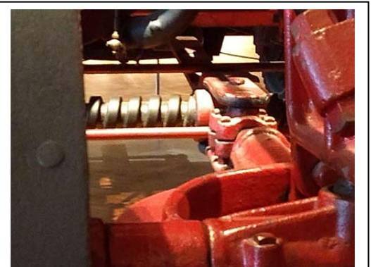
View looking over the front axle back to the steering worm. A "peg" block (red) surrounds the worm and moves side to side by the force of the Archimedes' screw.
