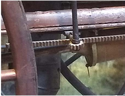
Rack and Pinion Steering from 1865!
