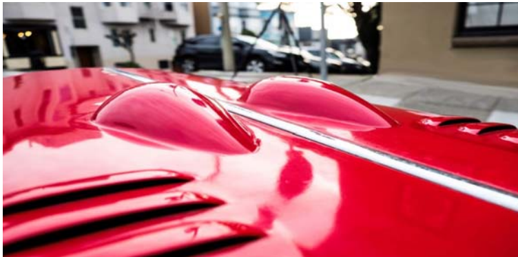
The SU dashpot-clearing bonnet bulges that called to mind a famously endowed country singer, inspiring Dolly's name.
