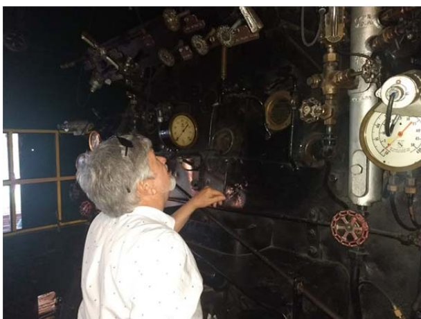
My brother Patrick checks out the gauges and controls of the 1941 Allegheny Locomotive, while I explained the operation of the boiler. One of the largest locomotive designs built, they weighed 604 tons, could pull a string of coal cars 1.25 miles long and do 60 mph!
