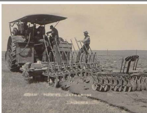
A steam traction engine at work pulling a ten-gang plow and a disc harrow; prepping a field for planting.
