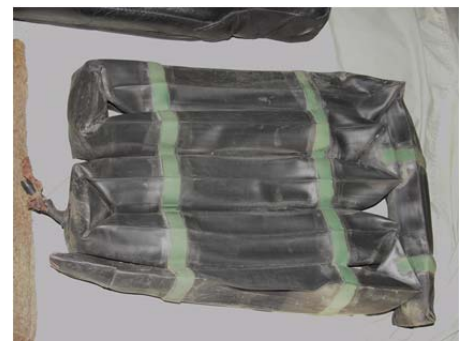
The air bladder for early Morgan seats that supports you and protects your hinny from the road bumps.
