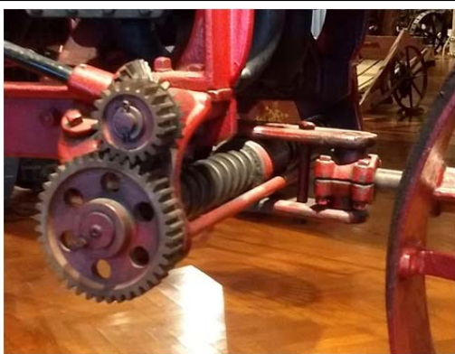
Bevel gears, straight cut reduction gears, large worm shaft and pinion type steering! This is on a 1916 Avery Traction Engine.
