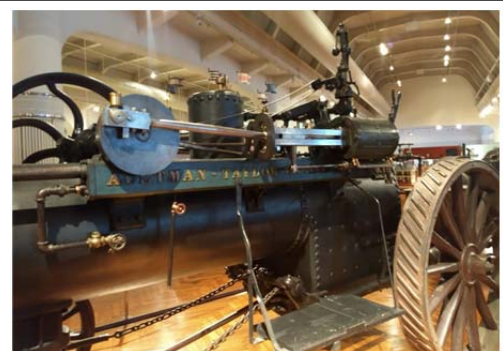
1886 Aultman-Taylor. Note the steering chains under the boiler.
