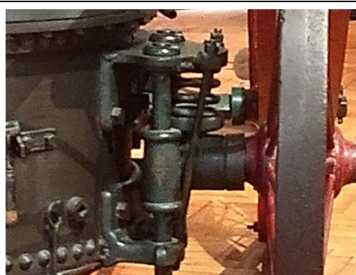
Sliding pillar suspension of 1881. This one uses two pillars for the "slide" as movement is only up and down with no pivoting involved.
