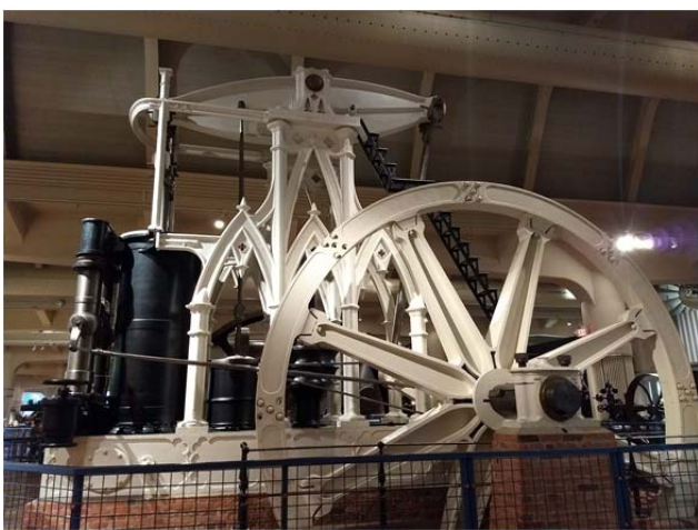
Industrial machinery as artwork! Note the gothic influence to this 1855 steam engine's frame.
