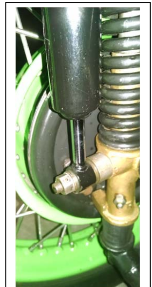
Only difference from 1881 is that this 3-Wheeler's sliding pillar rotates around the pillar to provide steering and it has a shock absorber.
